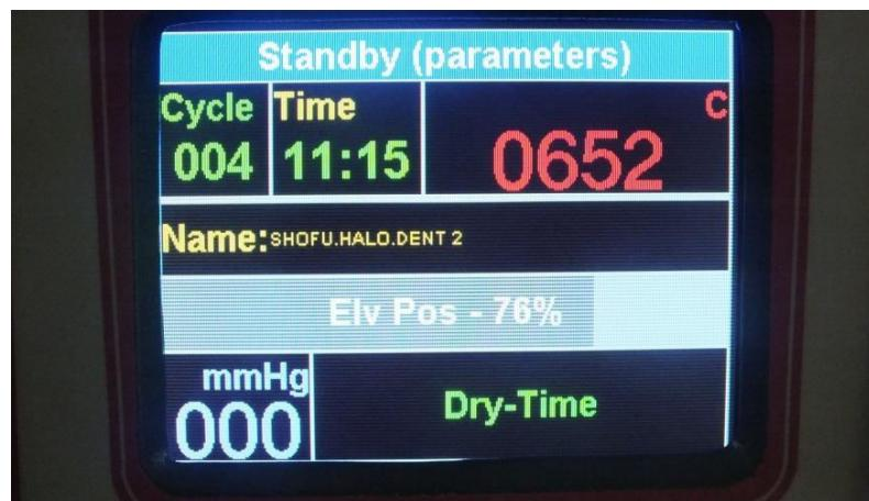
"Vacuum" display is used when keying in the vacuum parameters of the cycle. During the cycle, the "vacuum" screen is displaying the actual vacuum level on the lower left corner. **Lower left section**
